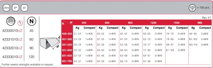
The above chart refers to chipboard or MDF 18 mm doors and aluminium frame doors with glass 4 mm thick.
